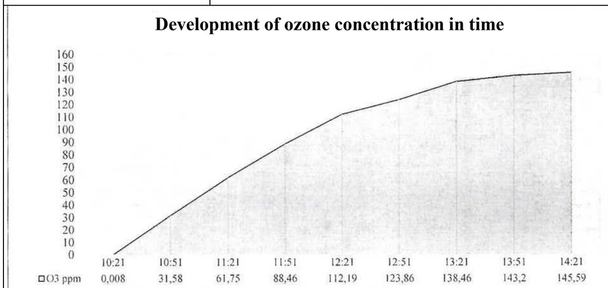
Figure 2 – Development of ozone concentration in the atmosphere of the test room
