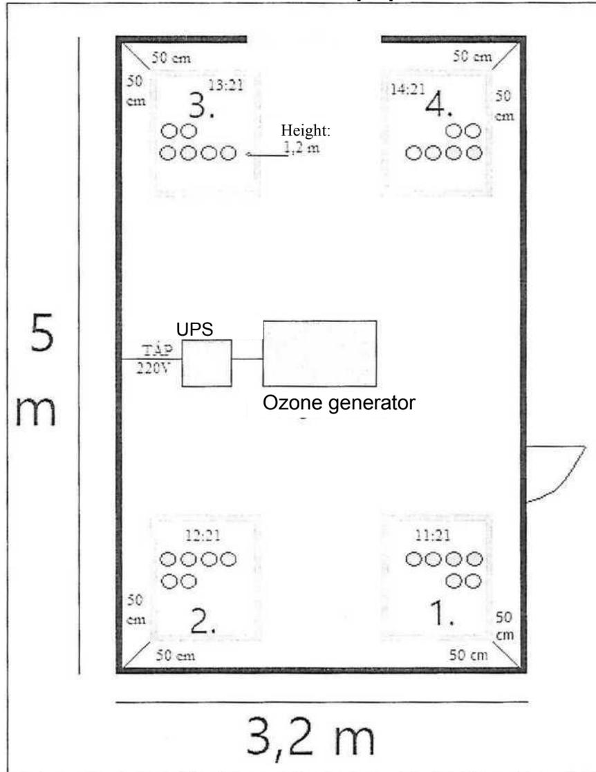
Figure 1 – Schematic layout of the test room – Drawing made by us.
